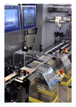
If the 2D code is incorrect, the affected folding box is removed from the production line at this point.
