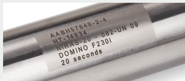
Waveform 0 can be used for engraving which is ideal for metals
