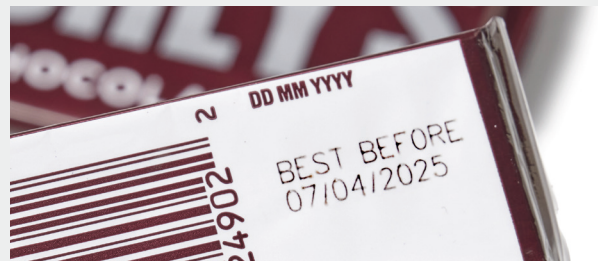
Waveform 2 creates a colour change which is ideal for foils
